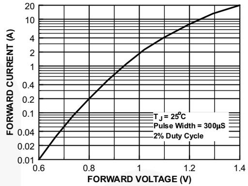
Figure 2. Forward Characteristics
