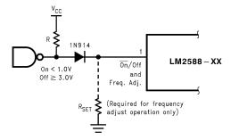
Figure 20. Shutdown Operation
