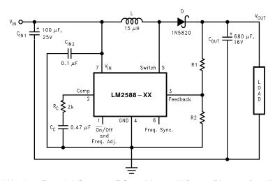
$C_{IN1}$ —100 μF, 25V Aluminum Electrolytic $C_{IN2}$ —0.1 μF CeramicL—15 μH, Renco #RL-5472-5D—1N5820 $C_{OUT}$ —680 μF, 16V Aluminum Electrolytic $C_C$ —0.47 μF CeramicR $_C$ —2kFor 12V Devices: R1 = Short (0 $\Omega$ ) andR2 = OpenFor ADJ Devices: R1 = 48.75k, ±0.1% andR2 = 5.62k, ±0.1%
