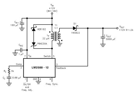
As shown in Figure 16, the LM2588 can be used as a flyback regulator by using a minimum number of external components. The switching waveforms of this regulator are shown in Figure 18. Typical characteristics observed during the operation of this circuit are shown in Figure 19.
