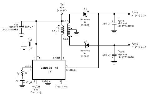
Figure 28. Dual-Output Flyback Regulator
