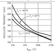
Figure 15. Oscillator Frequency vs Resistance
