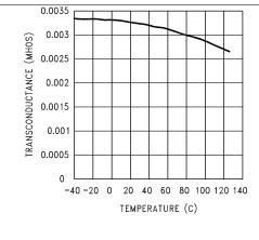
Figure 10. Error Amp Transconductance vs Temperature
