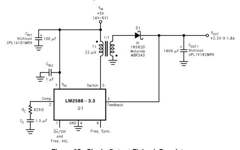
Figure 25. Single-Output Flyback Regulator
