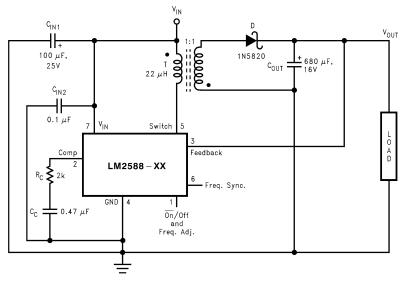
$C_{IN1}$ —100 μF, 25V Aluminum Electrolytic $C_{IN2}$ —0.1 μF CeramicT—22 μH, 1:1 Schott #67141450D—1N5820 $C_{OLIT}$ —680 μF, 16V Aluminum Electrolytic $C_{C}$ —0.47 μF CeramicR $_{C}$ —2k
