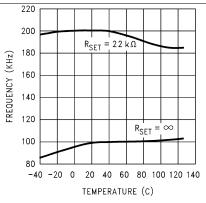
Figure 9. Oscillator Frequency vs Temperature
