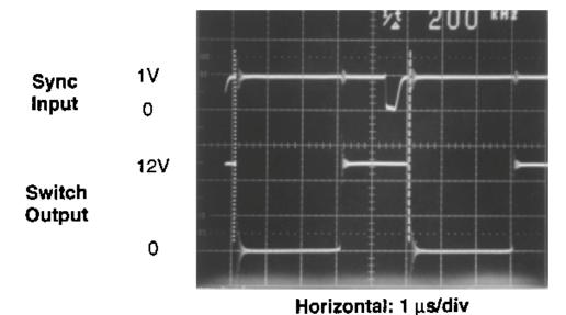
Figure 22. Waveforms Of A Synchronized 12-V Boost Regulator
