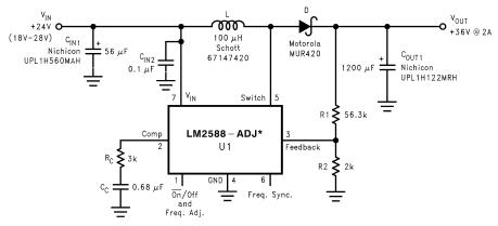
Figure 52. 24-V to 36-V Boost Regulator
