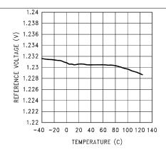
Figure 2. Reference Voltage vs Temperature
