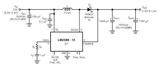
Figure 50. 5-V to 12-V Boost Regulator
