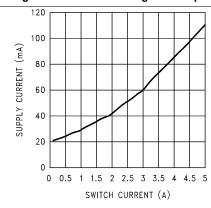
Figure 4. Supply Current vs Switch Current
