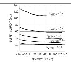
Figure 1. Supply Current vs Temperature
