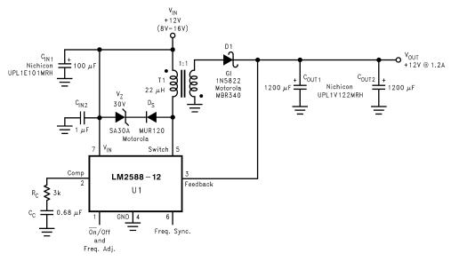
Figure 27. Single-Output Flyback Regulator
