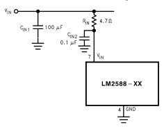
Figure 49. Input Line Filter
