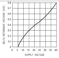
Figure 3.  $\Delta$ Reference Voltage vs Supply Voltage
