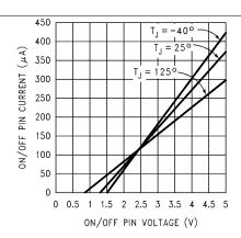
Figure 14. ON /Off Pin Current vs Voltage
