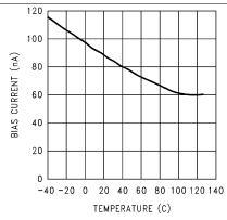
Figure 6. Feedback Pin Bias Current vs Temperature
