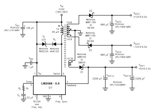
Figure 30. Triple-Output Flyback Regulator
