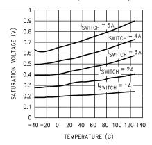
Figure 7. Switch Saturation Voltage vs Temperature
