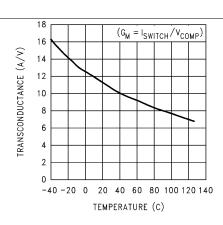
Figure 8. Switch Transconductance vs Temperature
