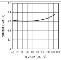
Figure 5. Current Limit vs Temperature
