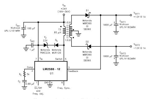
Figure 29. Dual-Output Flyback Regulator
