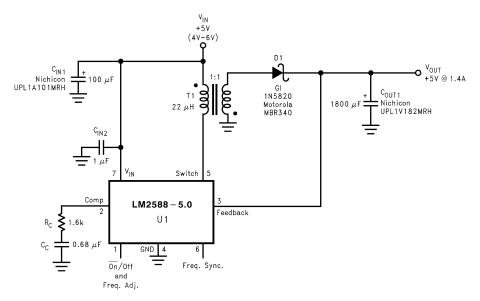
Figure 26. Single-Output Flyback Regulator
