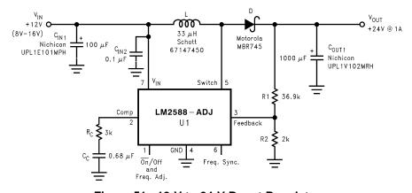
Figure 51. 12-V to 24-V Boost Regulator
