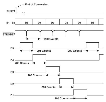
† Delay between BUSY going low and the first STROBE pulse is dependent upon the analog input.
