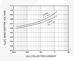
Figure 3. Base-Emitter Voltage
