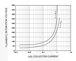
Figure 2. Collector-Emitter Saturation Voltage
